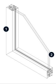
1 Aluminium profile with thermal break
